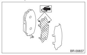
4) Install the brake pad to the support.
