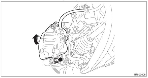
(3) Remove the brake pad from support.
