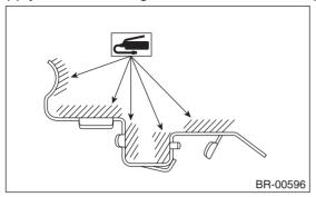
3) Apply a thin coat of Molykote AS880N (Part No. K0777YA010) or grease contained in the pad kit to both surfaces of the pad and inner shim.
