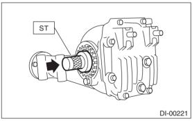
4) Install the rear differential. <Ref. to DI-28, IN-STALLATION, Rear Differential (T-type).> <Ref. to DI-45, INSTALLATION, Rear Differential (VA-type).>
