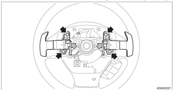
2) Disconnect the claws and then remove the lower cover.
