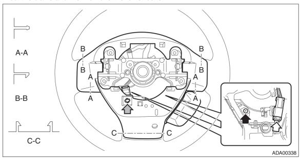
3) Remove the screw to remove the cruise control command switch assembly.
