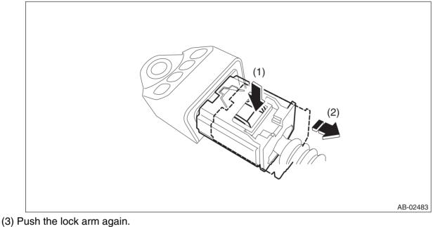
(4) Holding outer part, pull it in the direction of arrow to disconnect the connector.
