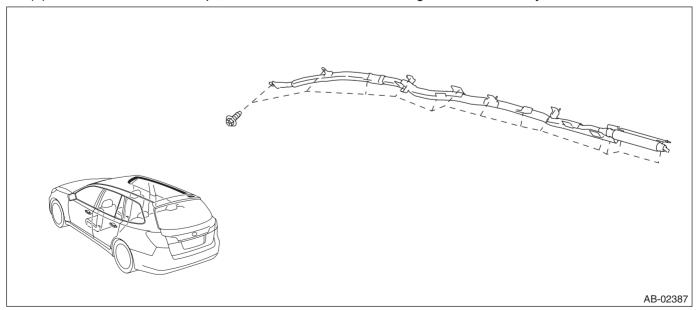
(2) Disconnect the curtain airbag module connector.
