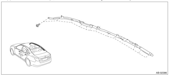
(2) Disconnect the curtain airbag module connector.
