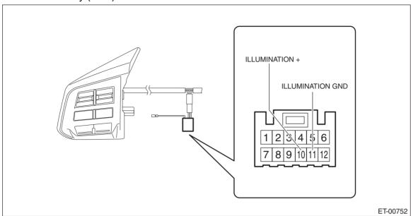
(2) If illumination does not turn on, replace the satellite switch assembly.
