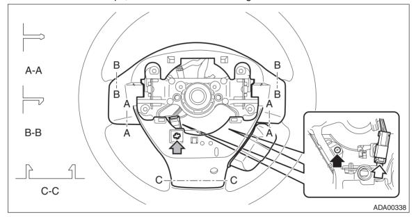
(4) Remove the screws and then remove the satellite switch assembly.
