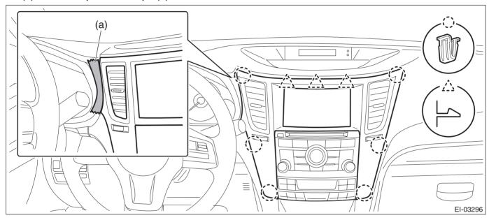
(2) Insert a finger into the air vent grille and release the left and right clips at the top of the center panel. (A), (B)
