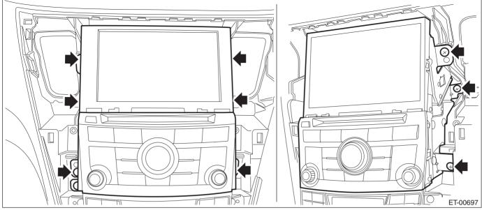
5) Remove the control panel assembly.
