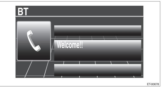
2) While "Welcome" is displayed, press "+"  $\rightarrow$  "HOOK OFF"  $\rightarrow$  "+"  $\rightarrow$  "HOOK OFF"  $\rightarrow$  "+" continuously in 5 seconds.
