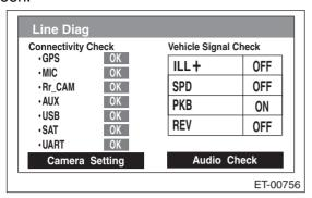
OK: Each connection device is connected properly.
