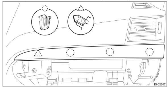
(4) Remove the screws and release the claws, then detach the glove box back panel.
