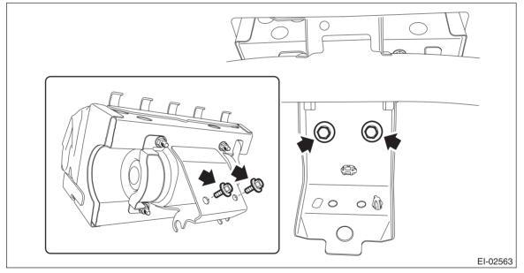
17) Remove the steering shaft assembly. <Ref. to PS-25, REMOVAL, Steering Column.>
