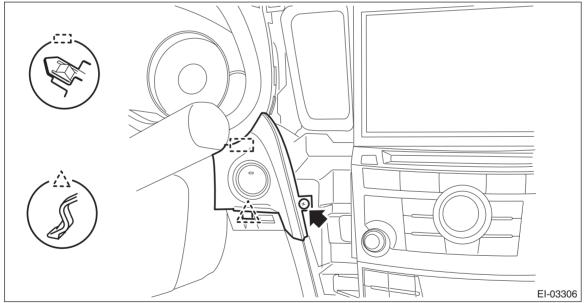
(2) Release the lock, tilt the steering column to the lowest end and fully extend the column by the telescopic system.
