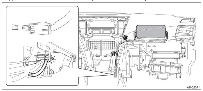
(2) Remove passenger's airbag module assembly bolts.
