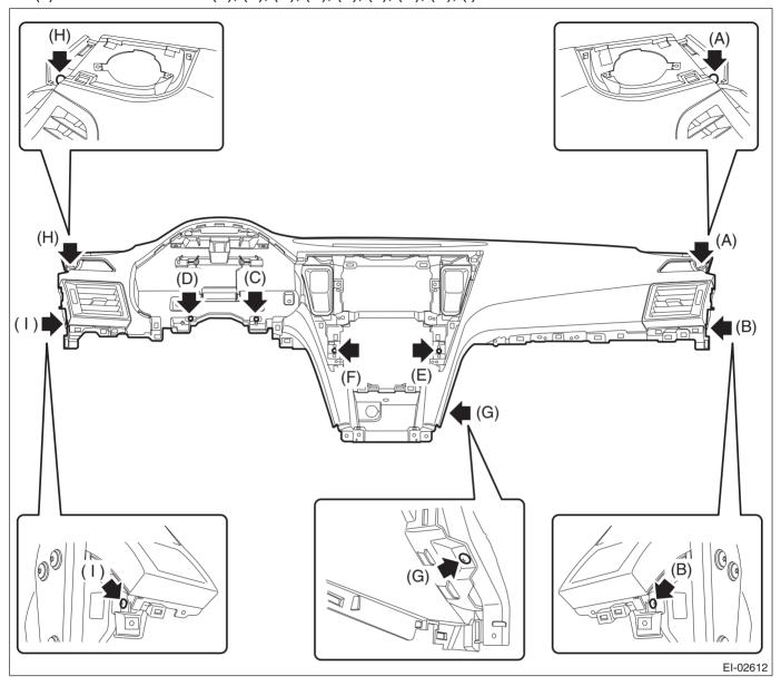
(2) Pull out the instrument panel assembly toward you and release the clamps of the left and right front side speakers.
