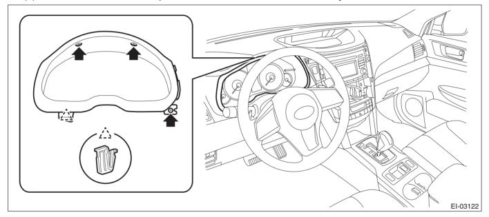
(4) Remove the screws and pull the steering COMPL upper cover toward you.
