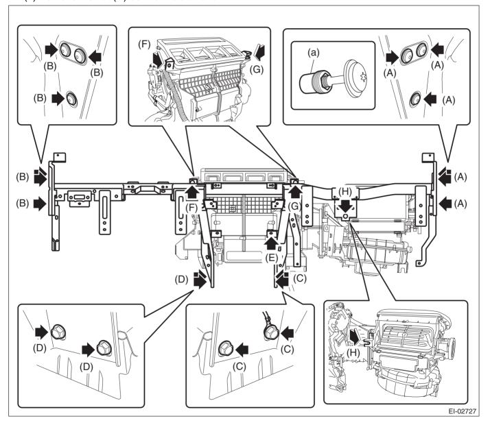
(8) Slightly lift the steering support beam assembly to detach the left and right pins. Then pull it toward you to remove the assembly.
