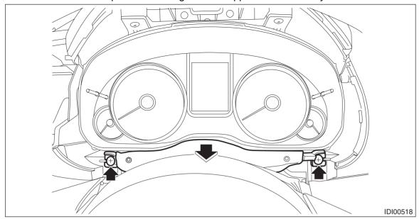
(5) Remove the four screws and pull out the combination meter toward you to disconnect the connectors.
