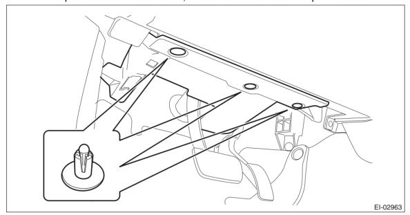
(3) Remove the screws and clips and release the claws, and remove the instrument panel lower cover while disconnecting the harness connectors.
