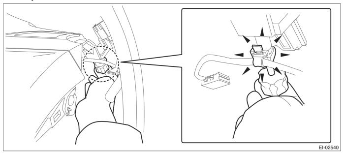
(3) After checking that all harness clamps and connectors are released and disconnected, remove the instrument panel assembly.
