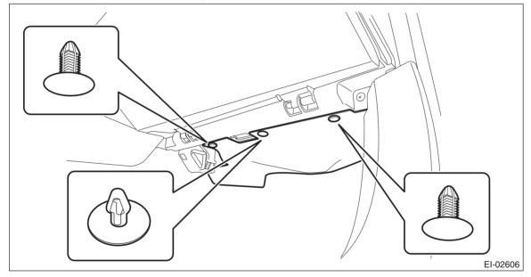
(3) Release the clips and claws, and remove the ornament panel assembly P.
