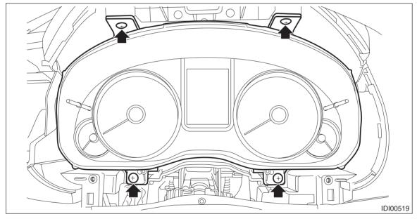
(6) Remove the combination meter assembly as shown in the figure.
