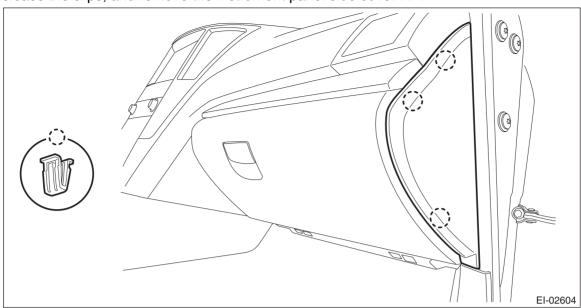
(2) Release the clips, and remove the glove box under cover.
