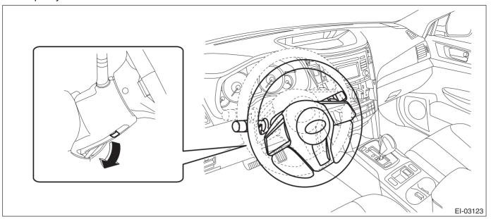
(3) Release the screws and clips, then detach the meter visor assembly.
