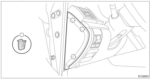
(2) Remove the clips and data link connector, and remove the instrument panel lower cover under.
