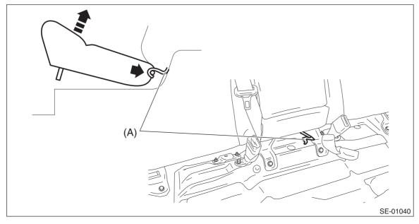
4) Release the clips and claws, and then remove the side sill cover - rear INN.
