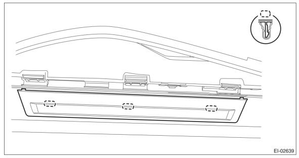
7) Release the claws and metal clips, and then remove the side sill cover-rear OUT.
