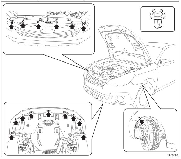
(6) Detach the flange section on the bumper face side from the bracket side front UPR.
