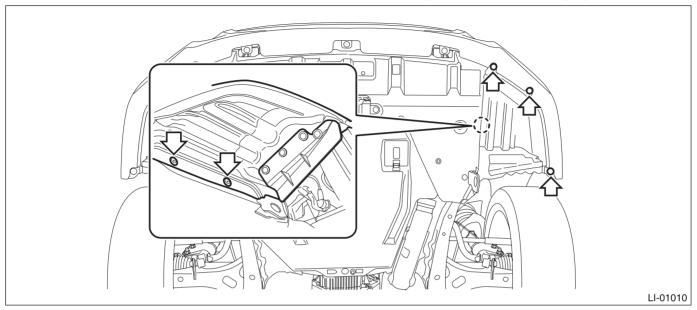
(2) Disconnect the front fog light connector. (Model with fog light)
