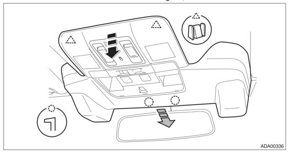
(5) Disconnect the connectors, and remove the stereo camera cover assembly.
