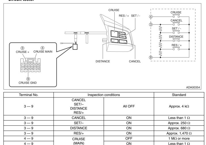
3) Replace the cruise control command switch if the inspection result is not within the standard.
