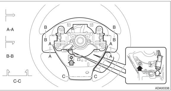
(4) Remove the screw to remove the cruise control command switch assembly.
