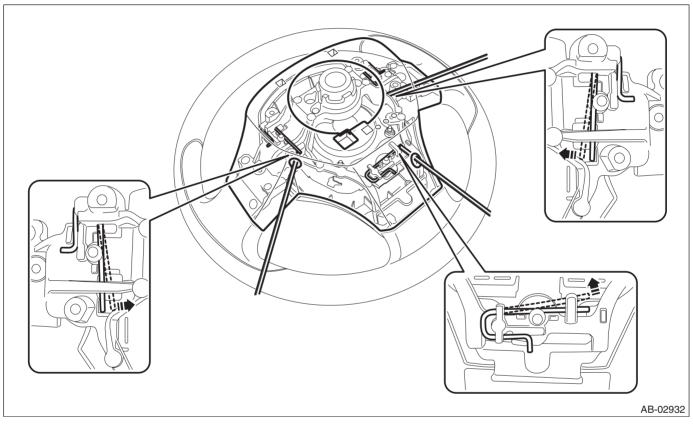
(2) Disconnect the horn harness and airbag connector and remove the airbag module assembly. <Ref. to AB-22, DRIVER'S AIRBAG MODULE, CURTAIN AIRBAG MODULE, PRETENSIONER & LAP SEAT BELT PRETENSIONER, PROCEDURE, Airbag Connector.>
