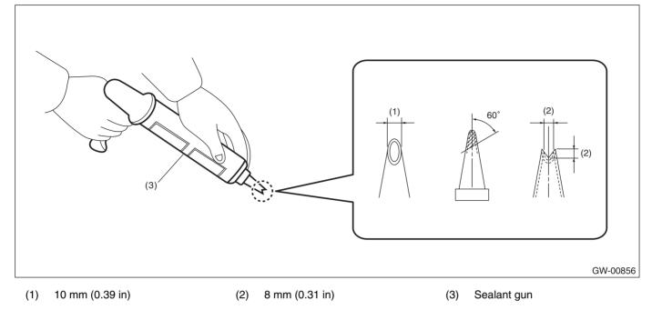
2) Prepare and clean the adhesion surfaces of the glass and body using the same procedures as for the windshield glass. <Ref. to GW-39, INSTALLATION, Windshield Glass.>
