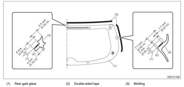
5) Install the rear gate glass in the same procedure as for windshield glass. <Ref. to GW-39, INSTALLA-TION, Windshield Glass.>
