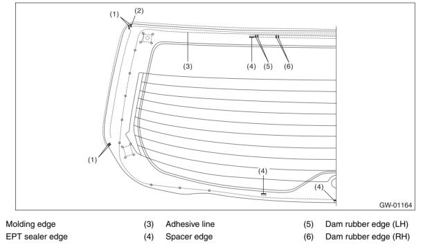
1) Fabricate the cartridge nozzle tip as shown and set the sealant gun with the adhesive.
