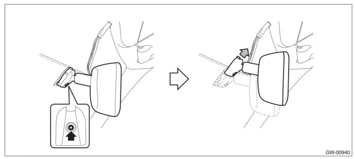
3) If the mirror mounting is damaged, replace the windshield glass.
