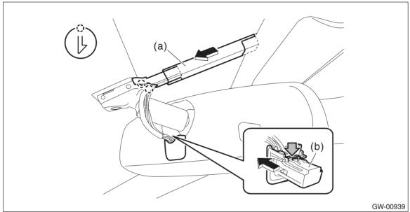
(3) Remove the TORX® bolt, and then slide the rear view mirror to remove.
