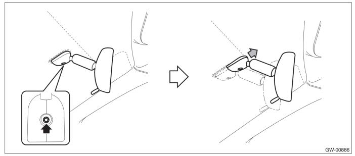
2) If the mirror mounting is damaged, replace the windshield glass.
