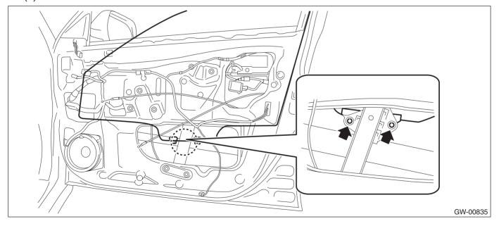
(3) While tilting the glass, remove the windshield glass.
