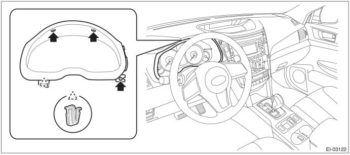
6) Remove the combination meter assembly.
