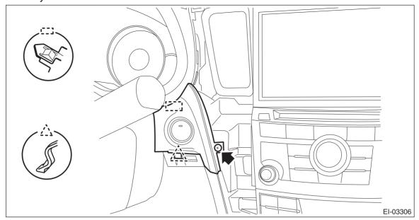
4) Release the lock, tilt the steering column to the lowest end and fully extend the column by the telescopic system.
