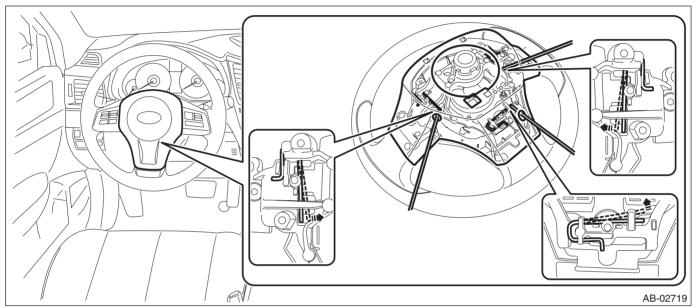
(2) Disconnect the horn harness and airbag connector and remove the airbag module assembly. <Ref. to AB-19, PROCEDURE, Airbag Connector.>
