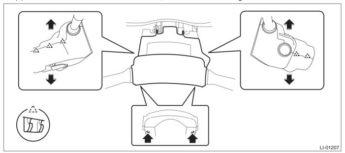
(3) Separate the steering column upper cover and steering upper cover, and remove the steering column upper cover.
