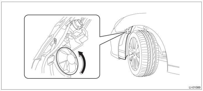
(2) Unlock the bulb socket and bulb spring, and remove the headlight low beam bulb.
