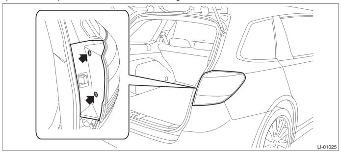
3) Remove the rear combination light assembly.
