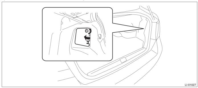
3) Remove the bulb socket and rear turn signal light bulb.
