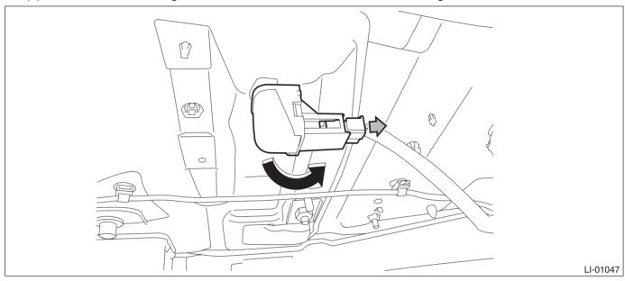
3) Release the claws, and detach the trunk room light cover and bulb.
