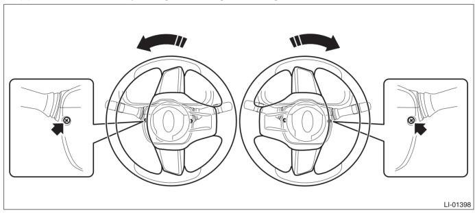
(2) Release the claws and remove the steering column lower cover.
