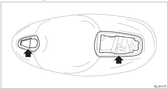
(2) Remove the TORX® bolt and remove the frame assembly from the door panel.
