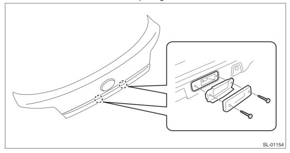
(5) Remove the license plate light assembly harness from the rear gate garnish.
