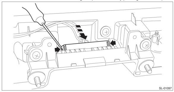
(2) Remove the screws and remove the rear lock button (lock). (model with keyless access)
