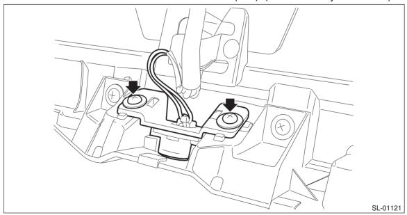
(3) Disconnect the rear exterior antenna connector. (model with keyless access)
