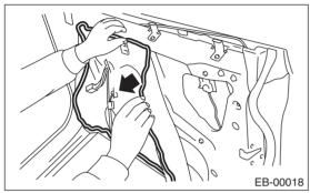
4) Remove the rod from the outer handle rod clamp.
