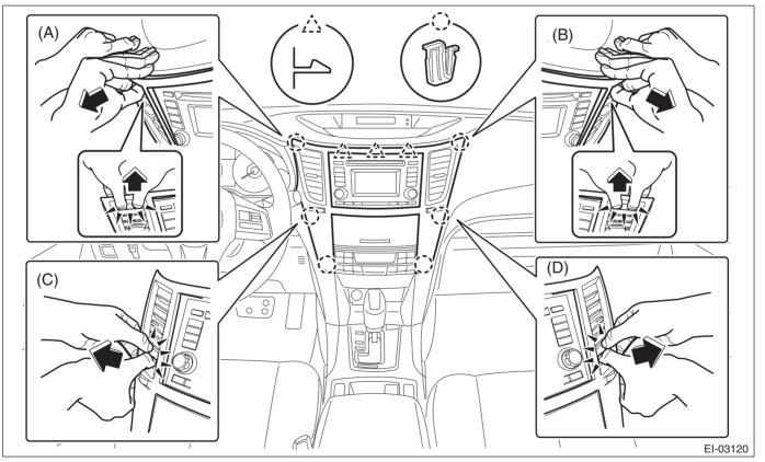
3) Remove the screws and release the claws, then detach the starter cover assembly.
