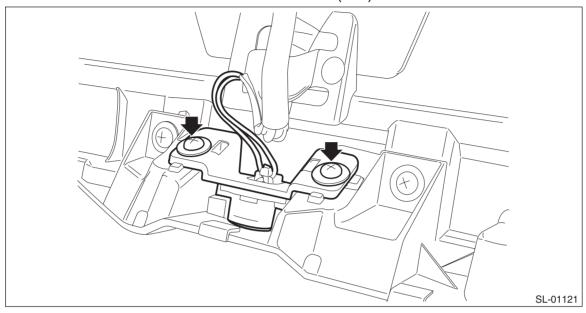
(2) Release the locks at both ends of the rear gate opener button by pushing with a flat tip screwdriver.
