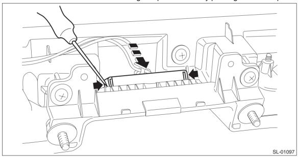
(3) Disconnect the rear exterior antenna connector.
