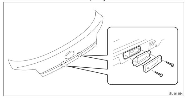
(5) Remove the license plate light assembly harness from the rear gate garnish assembly.
