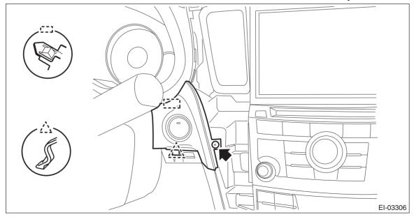
4) Release the claws and remove the push button ignition switch from the starter cover assembly.
