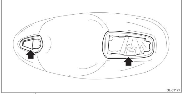
(2) Loosen the TORX<sup>®</sup> bolt and remove the frame assembly from the door panel.
