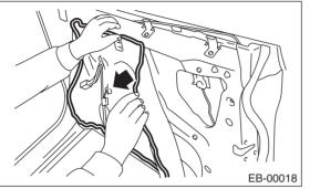
4) Remove the rod from the outer handle rod clamp.
