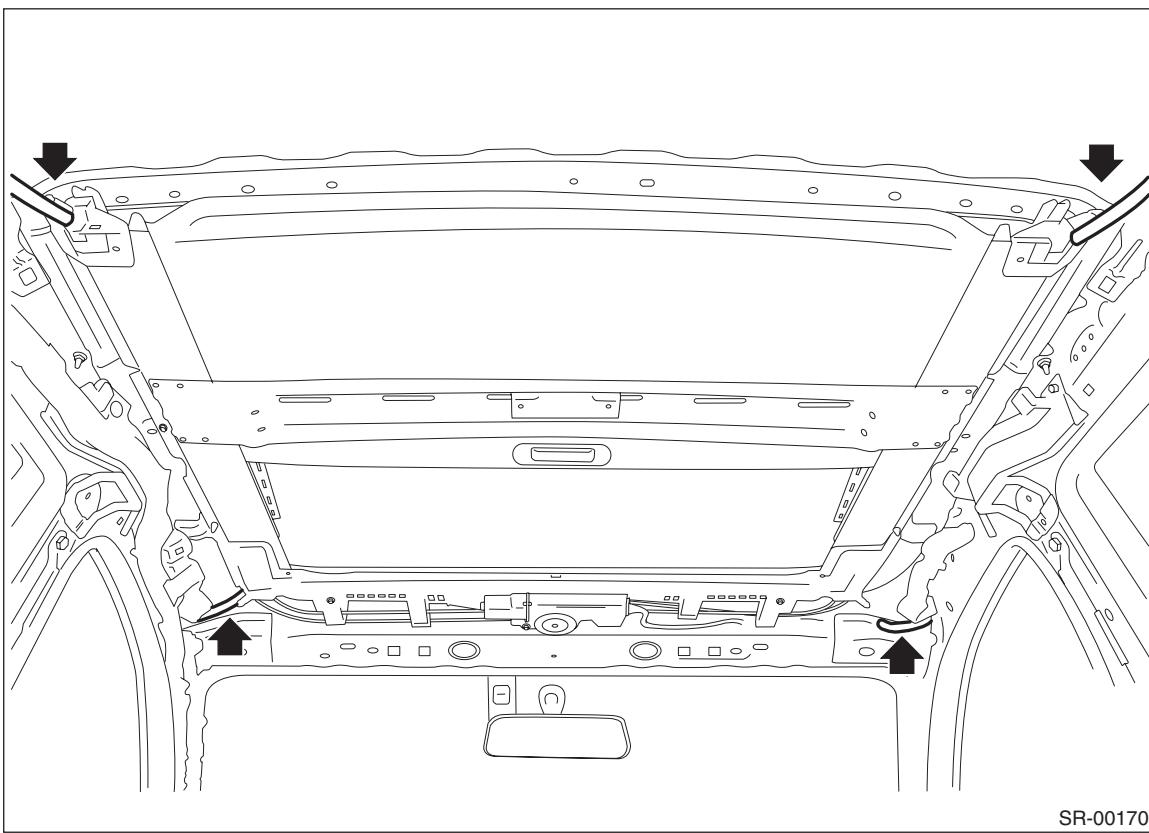
(2) Remove the bolts and then remove the sunroof bracket.
