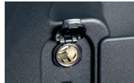
62 Cargo socket kit H6710AG000 Convenient 12-volt power outlet for outdoor activities etc.
