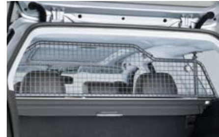
51 Dog guard (G/M) F551EAG011 Separates cargo room from passenger area, applicable for ISOFIX child seat.
