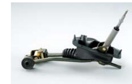
76 STI, Short gear shift lever (5MT, 6MT) C1010AG000, C1010AG100 Quick gear change and a more rigid & direct shift feeling. (Photo: 5MT) *Except for Dual-range transmission vehicle.
