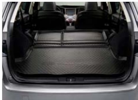
58 | Cargo Tray Foldable J515EAJ200 Like Cargo Tray, but foldable section covers rear seat back when laid down.
