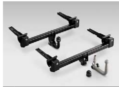
32 Trailer Hitch (Fixed, Detachable) L105EAJ600/L105EAJ610 L105EAJ700/L105EAJ710
