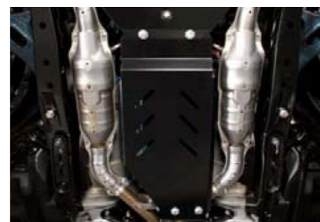
41 | Transmission Under Guard
