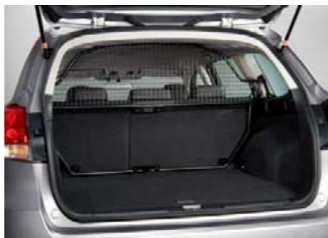
62 | Dog Guard (G/M) F555EAJ200 Equipped with a lower reinforcement brace for transporting large dogs.
