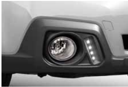
2 Daytime running lamps SENOAJ3001 Stylish and integrated LED lamps which improve driving safety without increasing fuel consumption. *Check availability with your dealer. OBR
