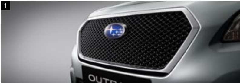
1 Front Grille J1010AL300 The resin-made grid mesh design gives a whole new image to the front.
