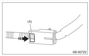
(2) With the slide lock pushed, disconnect the connector.
