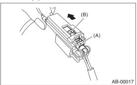
(3) While holding the slide lock in that position, release the lock arm (back to the original position), and disconnect the connector.
