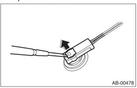
(2) Pull and disconnect the connector from the driver's airbag module assembly or retractor assembly.
