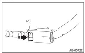
(2) With the slide lock pushed, disconnect the connector.
