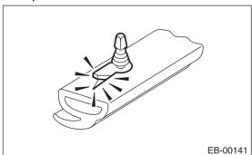
12) Remove the bolts and nuts to remove the door checker.
