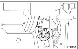
15) Put a wooden block on jack and place jack under the front door. Support the door with a jack to protect it from damage.
