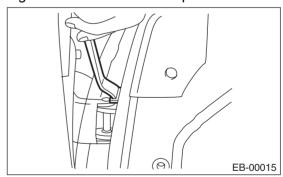
17) Remove the door hinge from vehicle.
