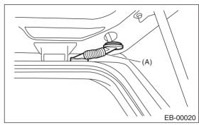
12) Before removing the rear gate damper stay, prevent the rear gate from closing using prop or the like.
