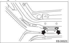
15) Remove the rear gate hinge from the vehicle.
