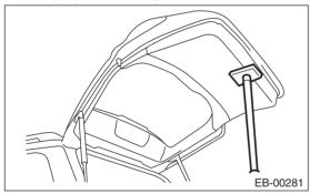
2) Remove the mounting bolt of rear gate damper stay.
