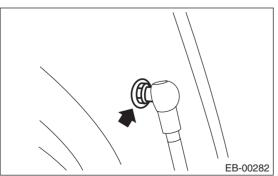
3) Remove the mounting bolts, and remove the damper stay.
