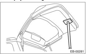
13) Remove the mounting bolt of rear gate damper stay.
