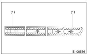
(1) Double-sided tape: Thickness = 1.2 mm (0.047 in) Width 5 mm (0.197 in)
