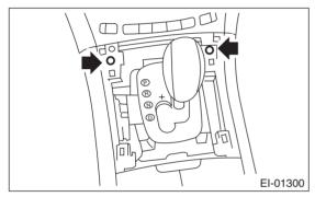
3) Remove the bolts inside the upper pocket.
