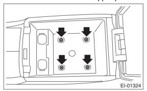
4) Pull out the console lower pocket, and remove the console box.
