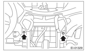
13) Make sure that the instrument panel upper is removed from the steering support beam
