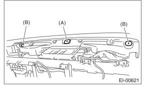
2) Check that the matching pins are inserted securely, and then route the harness.
