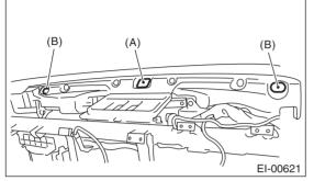
2) Check that the matching pins are inserted securely, and then route the harness.
