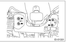
3) Remove the steering shaft from the steering support beam. <Ref. to PS-17, REMOVAL, Tilt Steering Column.>
