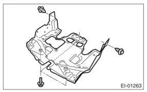
2) Remove the clips and bolts, then remove the front lower cover.
