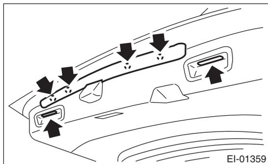
5) Remove the clips (A), and remove the rear gate lower trim.
