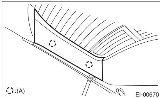
2) Remove the clips and claws (A), and remove the rear gate upper trim.
