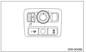
3) Remove the remote control mirror switch from instrument panel lower cover.
