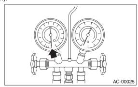
6) After 15 minutes of evacuation, if the reading shows 100.0 kPa (750 mmHg, 29.5 inHg) or higher, close the valves on the both sides to stop the vacuum pump.
