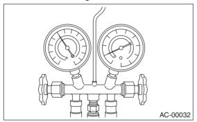
19) If the HFC-134a source is empty, close the high-pressure valve, close the valve on the can tap, and replace the HFC-134a source with a new part to restart the operation.
