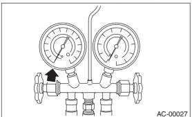
8) Leave it at least 5 minutes, and then check the low-pressure gauge reading for any changes. If the gauge indicator shows near zero point, it is a sign of leakage. Check pipe connector points, repair them, and make sure there is no leakage.
