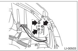
6) Remove the two bolts and then remove the headlight assembly.
