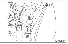
7) Disconnect the connector and then detach the rear headlight assembly.
