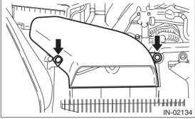
3) Remove the engine front cover.
