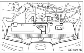
4) Disengage the three clips, and then turn over the mud guard.
