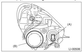
6) Remove the light bulb retaining spring (A) to remove bulb.
