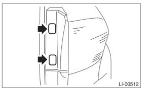
3) Remove the two bolts, and then detach the rear combination light by pulling it to the rear side of vehicle.
