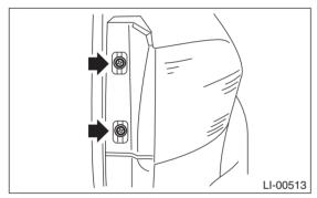
4) After turning the sockets of the tail/stop light bulbs and rear turn signal light bulbs, remove the rear combination light.
